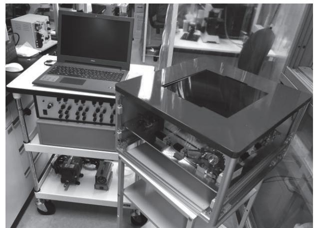
Fig.2 Prototype high-throughput screen planar patch clamp device.
