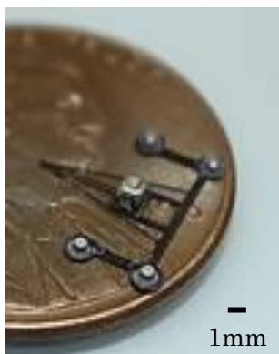
Fig.1 Micro-robot made of Si
