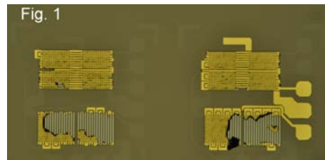
Fig. 1 Failure mode of AMR element.
