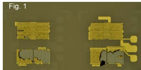
Fig. 1 Failure mode of AMR element.
