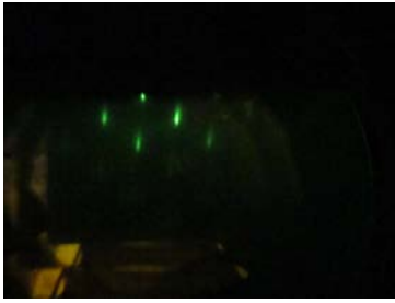
Fig.4. The surface shape after growing LT-GaAs at 300°C.
