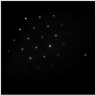
Fig. 5. TEM image of the electron diffraction pattern.
