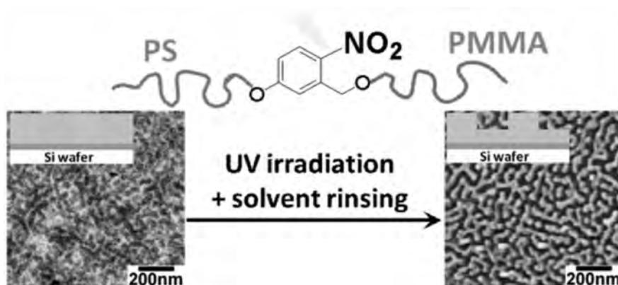
Figure 2. Simplified molecular image of PS-ONB-PMMA (top) and AFM images of PS-ONB-PMMA thin film before and after UV irradiation and selective solvent rinsing (bottom).
