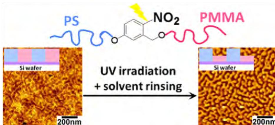
図2. Simplified molecular image of PS-ONB-PMMA (top) and AFM images of PS-ONB-PMMA thin film before and after UV irradiation and selective solvent rinsing (bottom). 研究成果報告 (1) より
